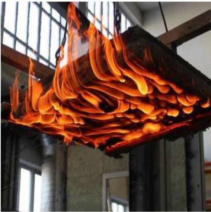
Three unloaded CLT panels were exposed to a standard fire test in fall 2018 in Zurich/Switzerland.
